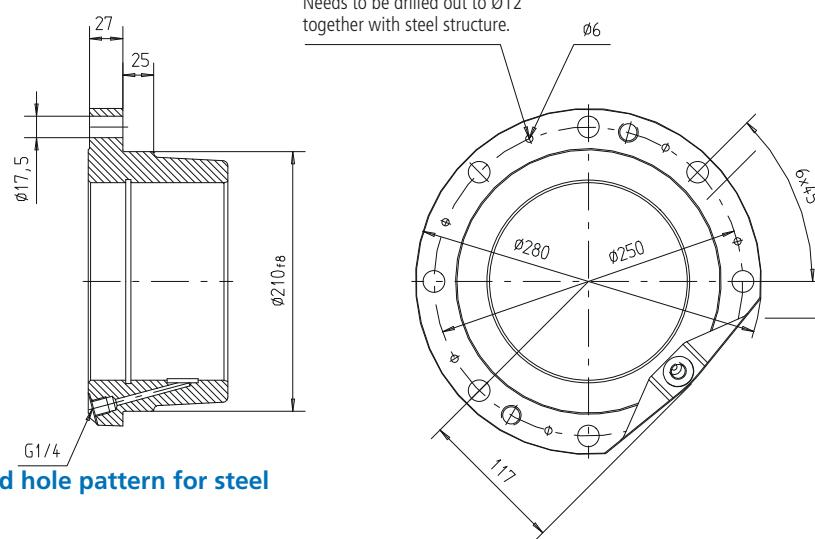
**Fitting dimensions and hole pattern for steel construction**
